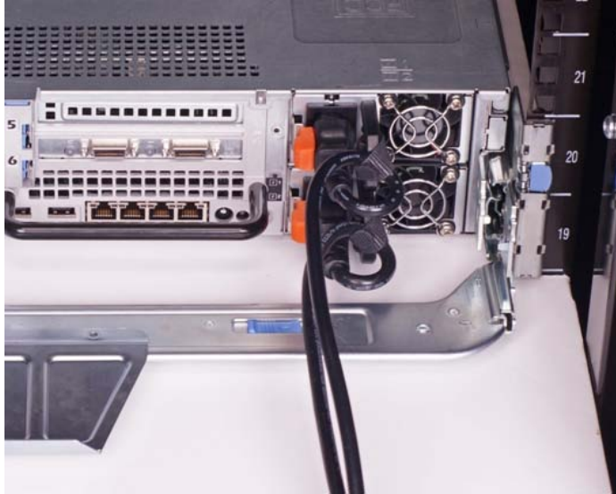
Figure 2: Routing Power Cables Through the Strain Reliefs
